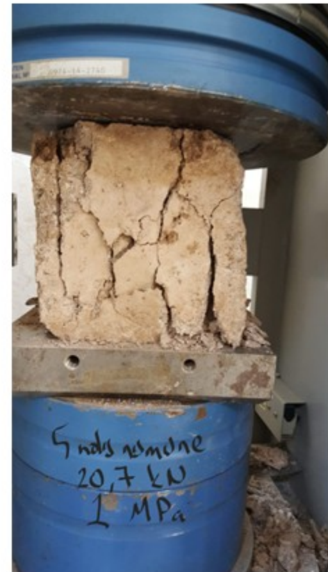
Soil samples were tested for compressive strength, Erzincan Binali Yıldırım University, 22 October 2020
