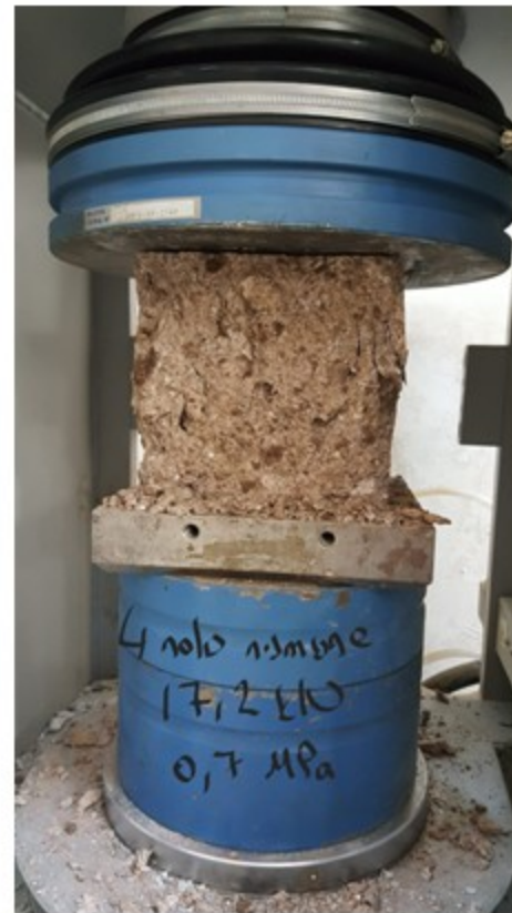
Soil samples were tested for compressive strength, Erzincan Binali Yıldırım University, 22 October 2020
