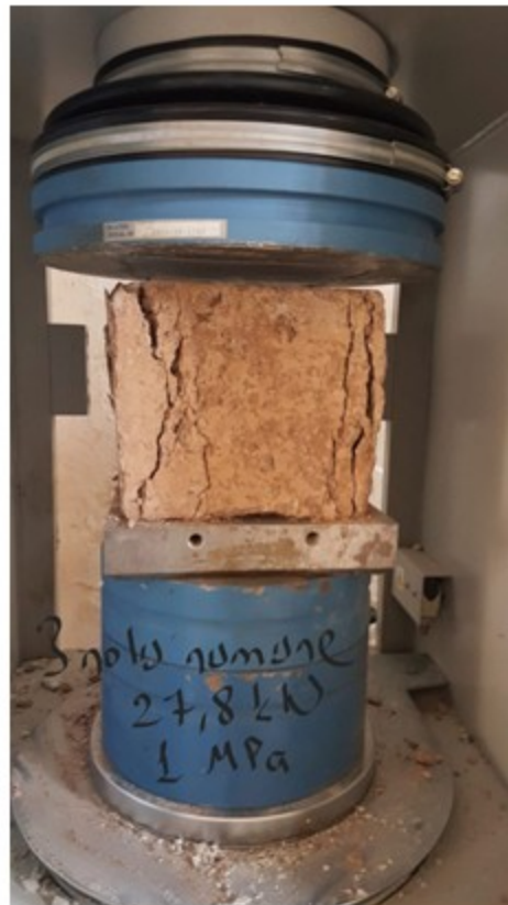
Soil samples were tested for compressive strength, Erzincan Binali Yıldırım University, 22 October 2020
