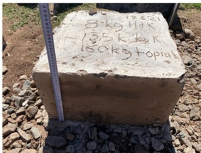
Soil mixture samples at different ratios were prepared and poured into the mold, 20 June 2021
