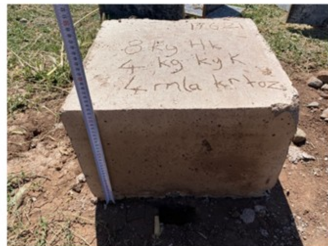
Soil mixture samples at different ratios were prepared and poured into the mold, 20 June 2021
