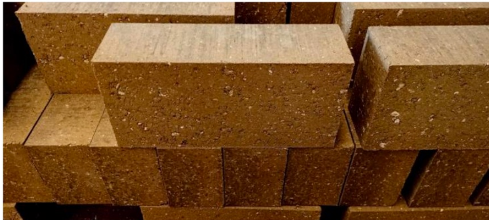
Figure 5. Compressed Earth Blocks made of excavated earth (Resource: URL 6)
