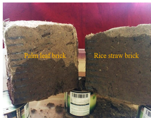
Figure 18. After 5 hours of the test, the Amount of water absorbed in both bricks. Author
