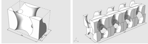
Figure 3. The single block form and assembly method of the blocks
