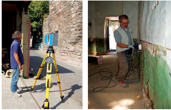
Figure 1.2. Photogrammetric drawings of the building, The georadar implementation to define the gaps on the walls and plastered surfaces
