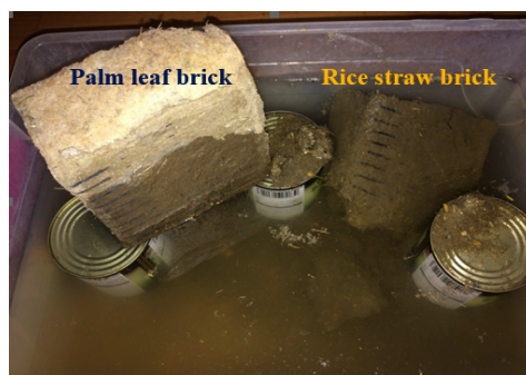
Figure 19. After 12 hours, the final result is the collapse of the rice straw Adobe brick, Author
