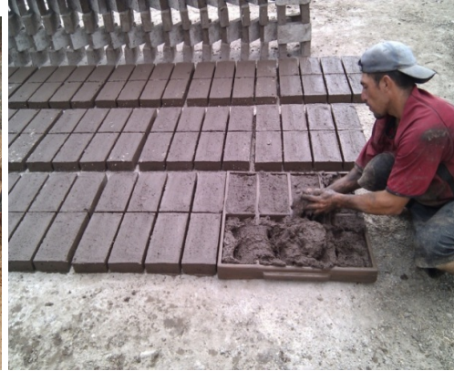
Figure 14. the framing process
