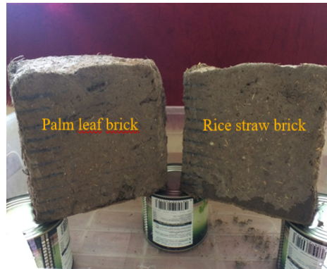
Figure 16. At the beginning of the test, comparing between two Adobe brick made of rice straw and palm leaf. Author
