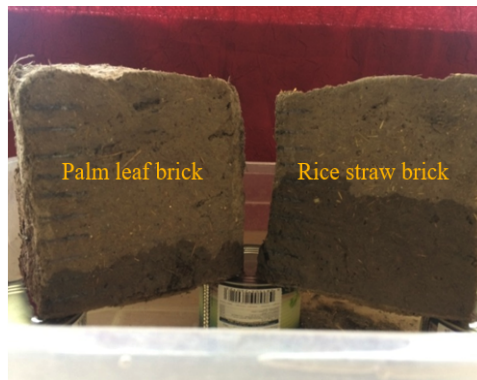
Figure 17. After an hour of the test, the Amount of water absorbed in both bricks. Author
