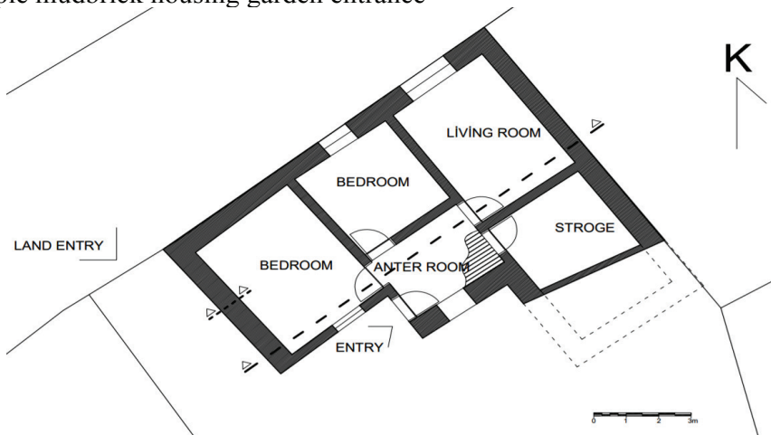
Figure 5. Sample mudbrick housing space distributions.
