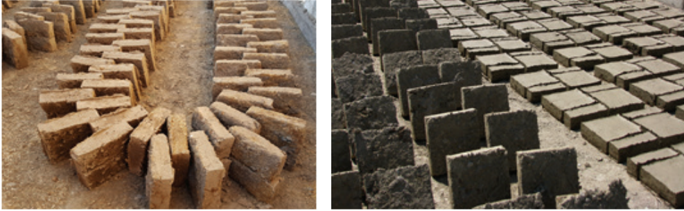
Photo 13, 14. Mud-Brick Drying Views (Ş. Öztürk)
