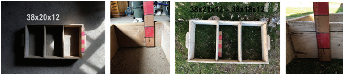
Figure 10. Adobe brick mold – type 1 and type 2
