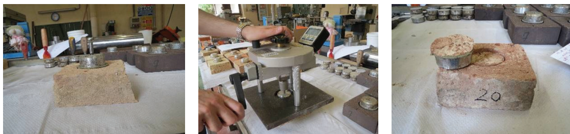
Figure 2. process of pull off test. Before (left) during (center) and after (right)
