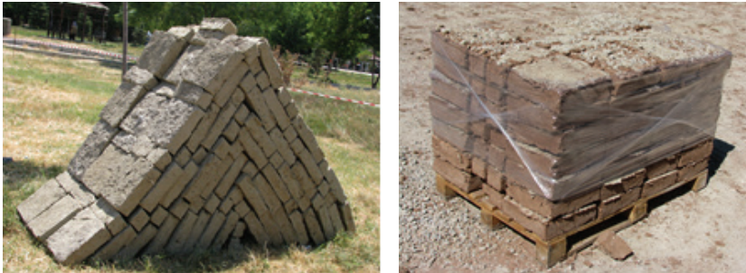
Photo 15, 16. Mud-Brick Stack And Packaging Views (Ş. Öztürk)
