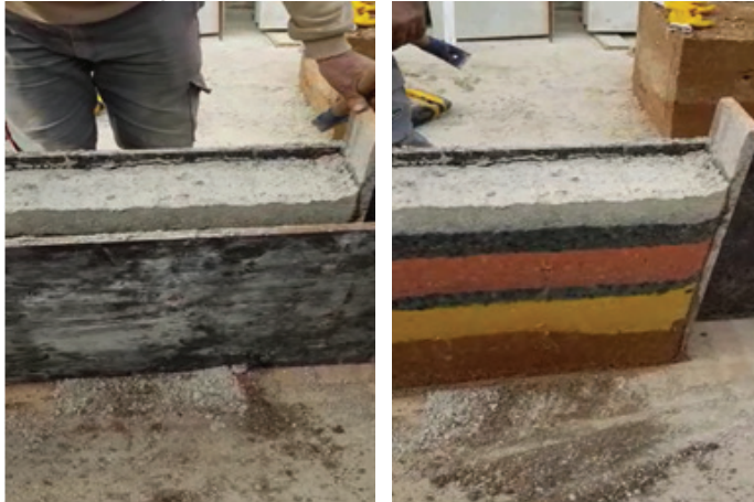
Figure 11. Samples of different colored rammed earth walls
