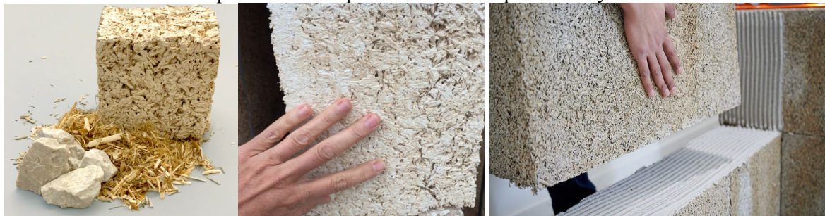
Figure 1. Hemp, lime and hempcrete [19]. Figure 2. Hempcret Block [20].
